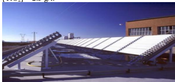
FIGURE 2. Pilot installation for water purification under sun light irradiation. 100 m 2 installed at HIDROCEN (Madrid, Spain).
