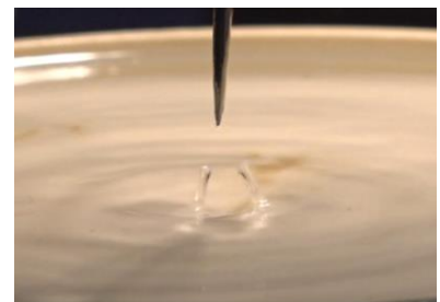
FIGURE 2. Columns above the surface of butyl glycol. Negative corona. The distance from the end of the needle to the surface of the liquid is 7 mm. V=10 kV.
