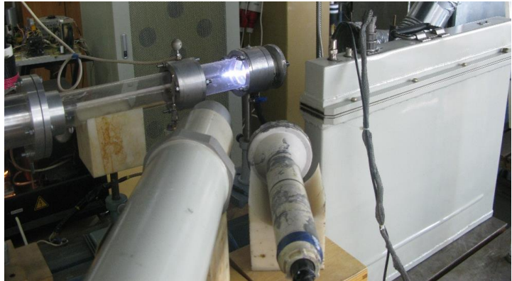
FIGURE 2. General view of the experimental set up PVR with detector CPIIC and radiometer KPAH-1
