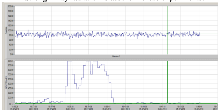
FIGURE 3. Neutron's signal (down) and \gamma -radiation signal (top) measured CPIIC-detector.
