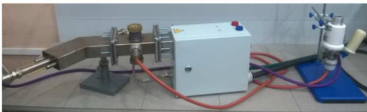
FIGURE 1. Sketch and a view of the microwave plasmatron with an external plasma torch [2, 4].
